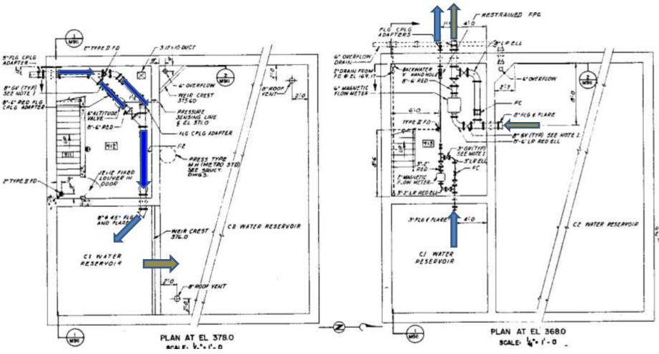
C1 Capacity – 171,000 gallons, 32'w x 52'l x 13.75'd – Q<sub>p</sub> =1,100 gpm C2 Capacity – 18,400 gallons, 12.16'w x 14' l x 14.5'd - Q<sub>p</sub> =100 gpm
