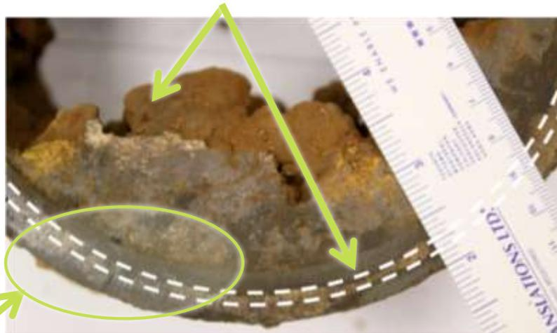
This is the remaining structural thickness!
