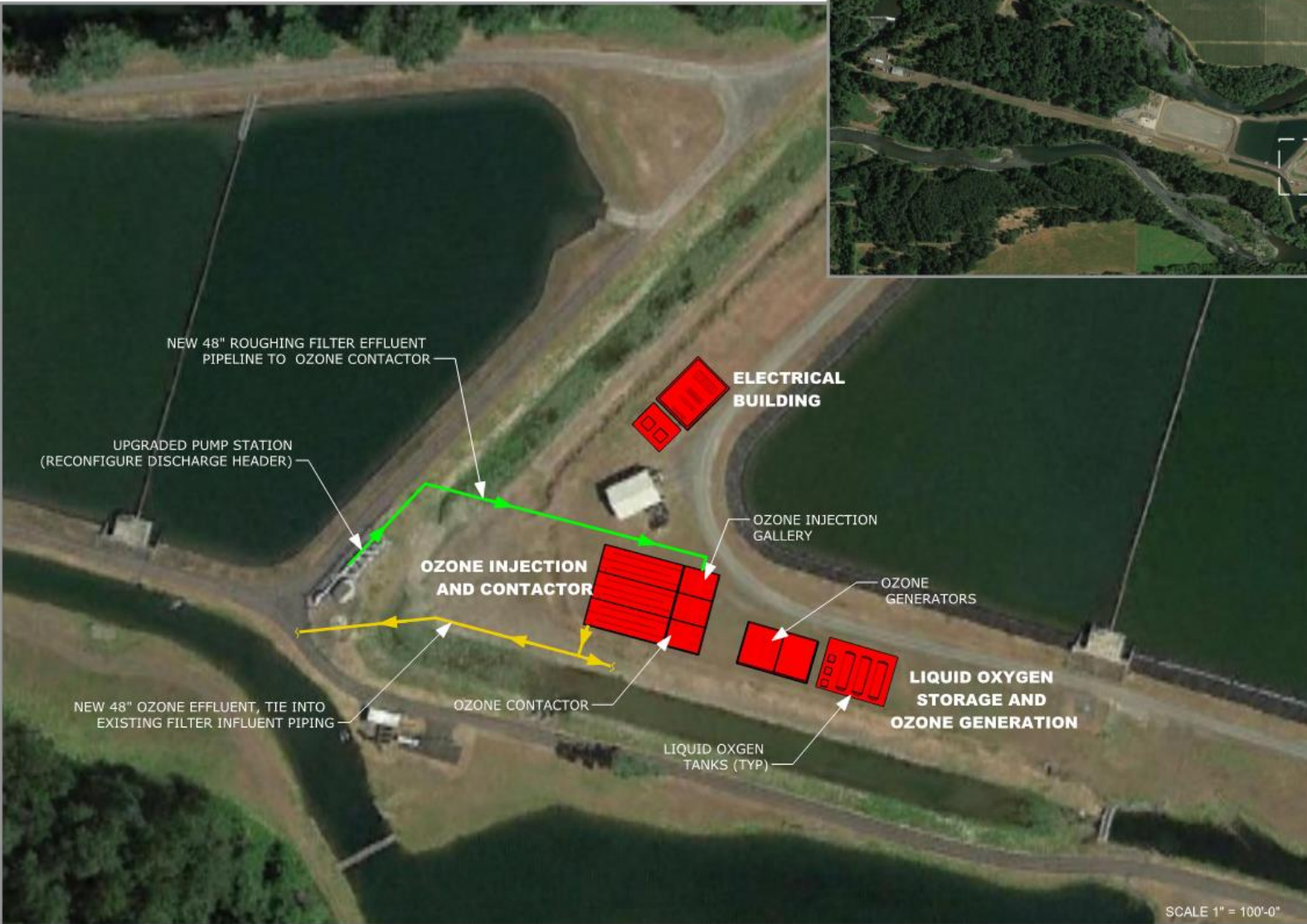
INTERMEDIATE OZONE CONCEPTUAL LAYOUT
