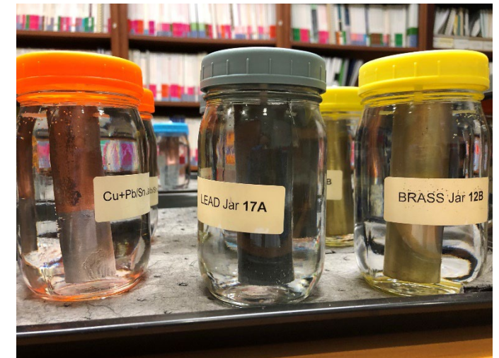
Copper, lead, and brass coupon jars about 6 weeks into acclimation in pH 8.5 test water.
