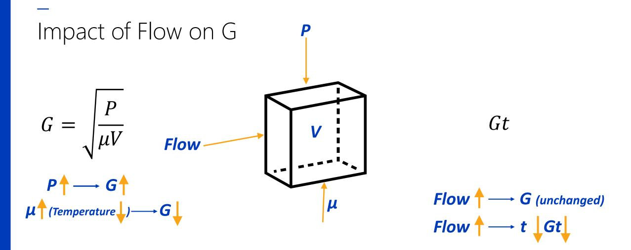
G = velocity gradient (s<sup>-1</sup>) P = Power of mixing input (kW / HP) V = Volume of mixing vessel (ft<sup>3</sup>, m<sup>3</sup>)  $\mu$  = Viscosity (N-s/m<sup>2</sup>, lb-s/ft<sup>2</sup>) G = velocity gradient (s<sup>-1</sup>) t = Mixing time (s)
