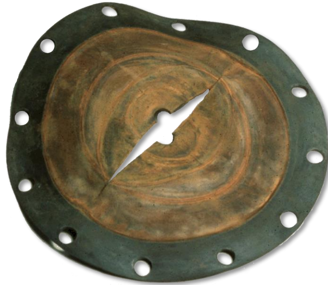
Diaphragm "whipped" – stem nut was not tight enough!
