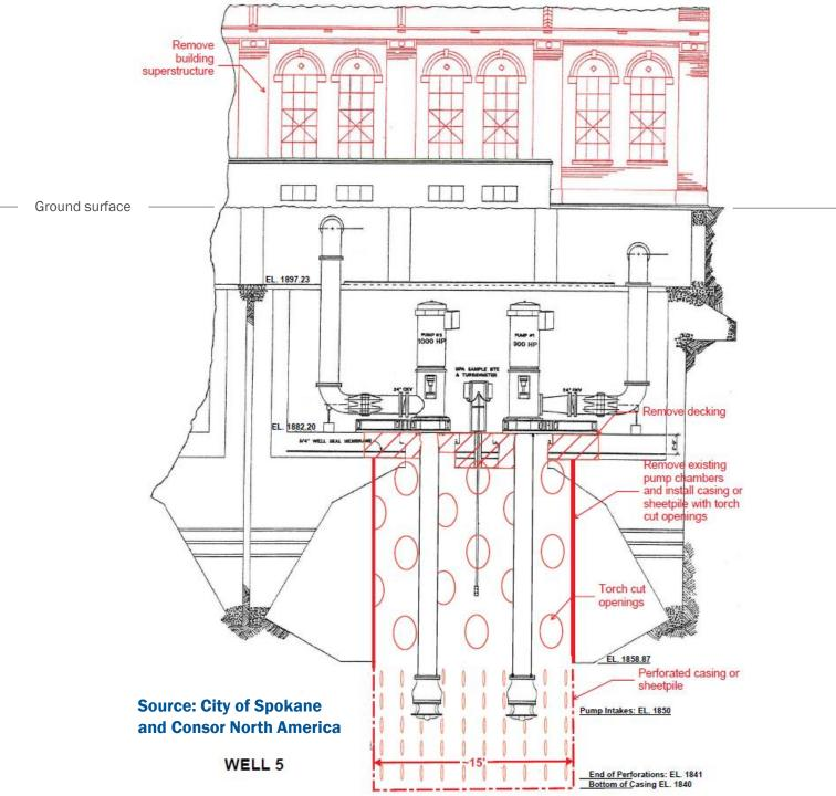
Alternative No. 2 – Install Pump Chamber
